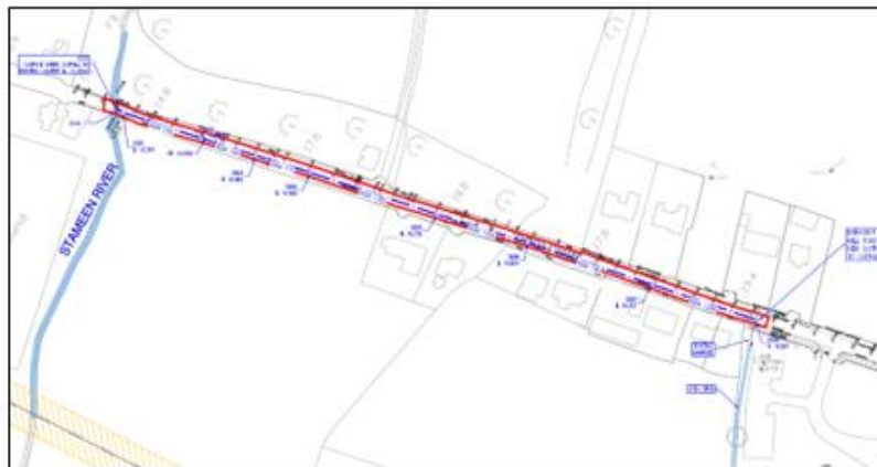
Figure 2: Extract of Surface Water Outfall Plan showing proposed surface water outfall pipe on Mill Road
